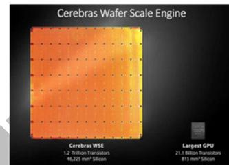
ii. This chip has **1.2 trillion transistors**, the basic on-off electronic switches that are the building blocks of silicon chips.
